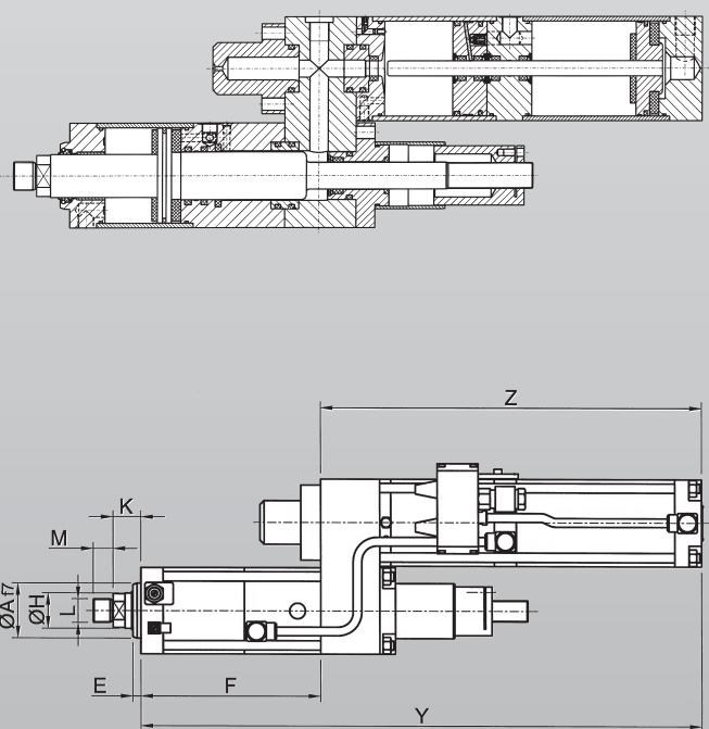
The measurements of the MULTIPOWER head piece are according to the mentioned data's of version G or U.
