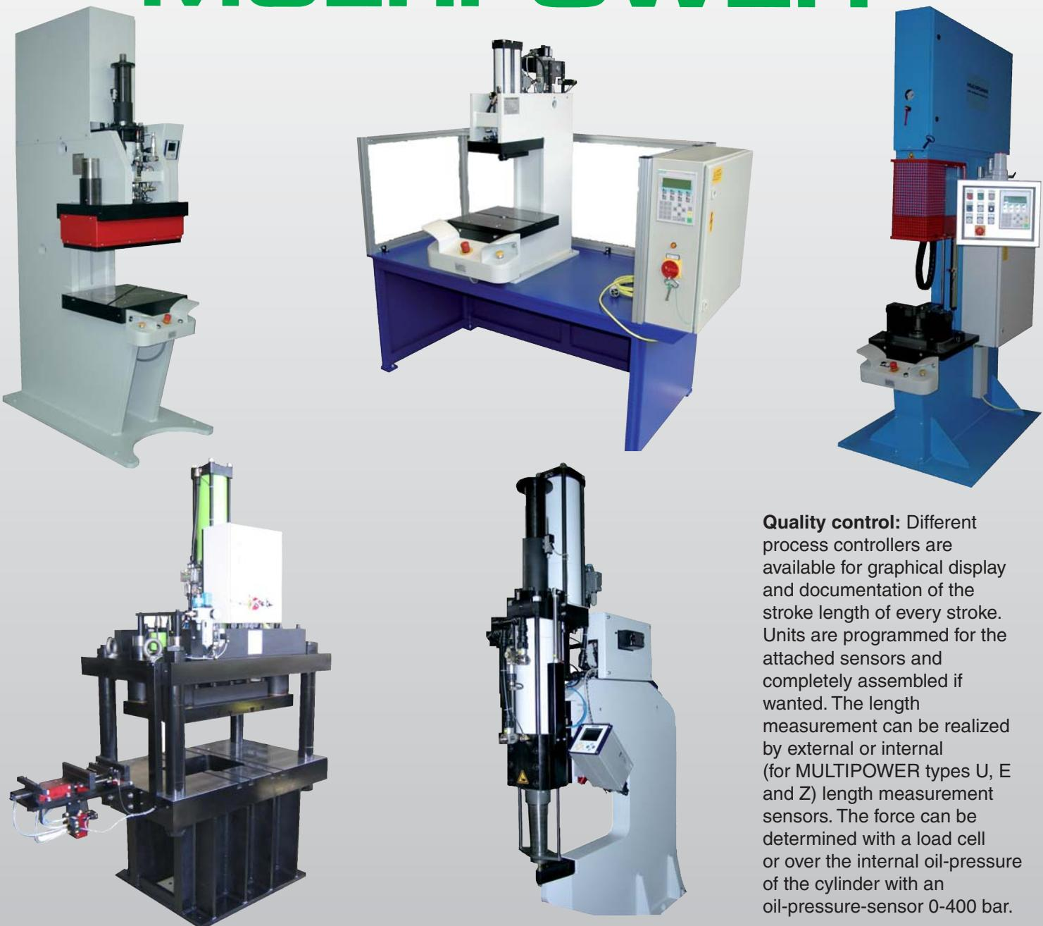
**Quality control:** Different process controllers are available for graphical display and documentation of the stroke length of every stroke. Units are programmed for the attached sensors and completely assembled if wanted. The length measurement can be realized by external or internal (for MULTIPOWER types U, E and Z) length measurement sensors. The force can be determined with a load cell or over the internal oil-pressure of the cylinder with an oil-pressure-sensor 0-400 bar.
